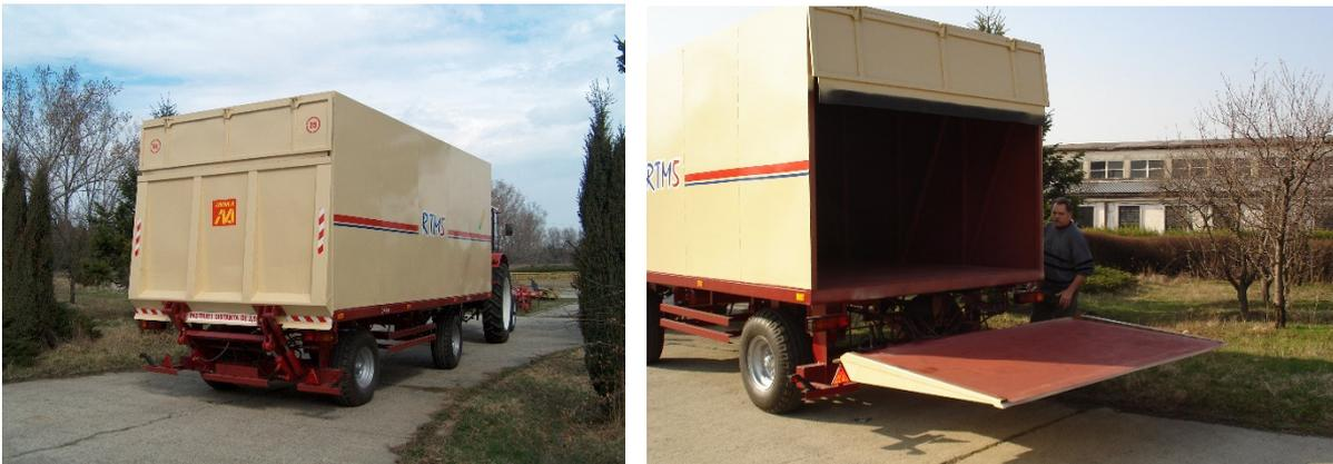
Fig. 1. Trailer with mobile shutter for transporting packed or containerised products made at INMA Bucharest – RTM5 [4]
